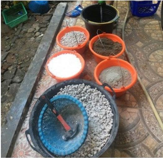
Gambar 5. Komposisi Material Sampel Uji (*Eco-brick*)
