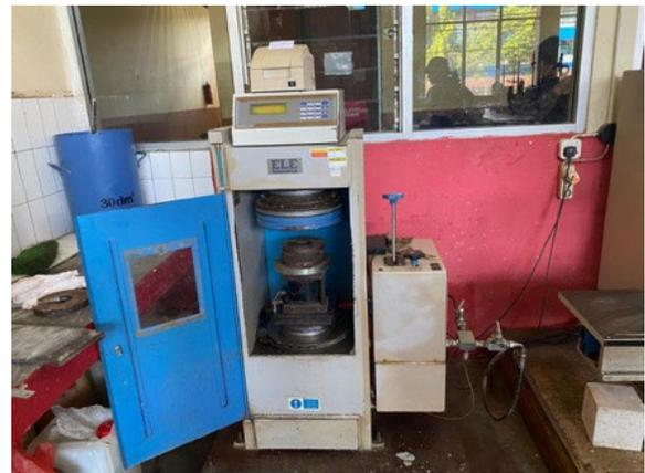
Gambar 8. Alat Uji *Compressive Strength*
