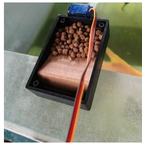
Figure 4. 3 Automatic Fish Feeding Using Servo Motor
