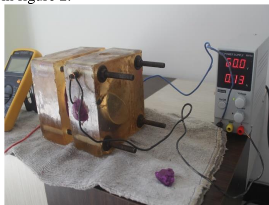
Figure 2. Rapid Chloride Penetration Testing Procedure
