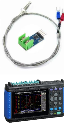
Figure 1. MAX6675 K-type thermocouple sensors and LR8432 heat flow logger
