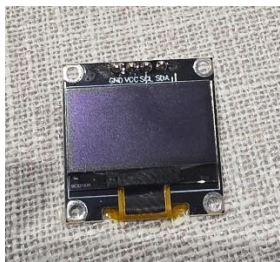
Figure 4. 0.96 Inch I2C OLED Display
