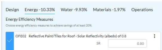
**Gambar 4. 3 Data Reflective Paint for Roof [8]**
