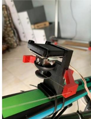
Figure 4.7 Analog Joystick Module Installed
