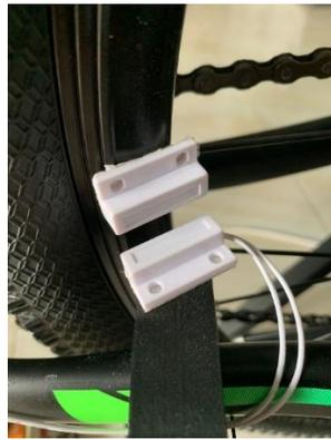
Figure 4.6 Magnetic Sensor Installed on the Bicycle
