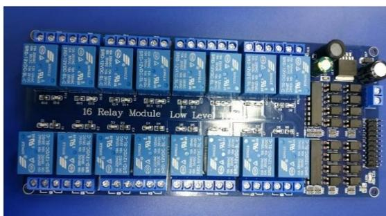
Figure 5. 16 Channels Relay
